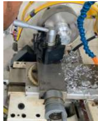
Gambar rajah 16. Proses boring tengah pinan
